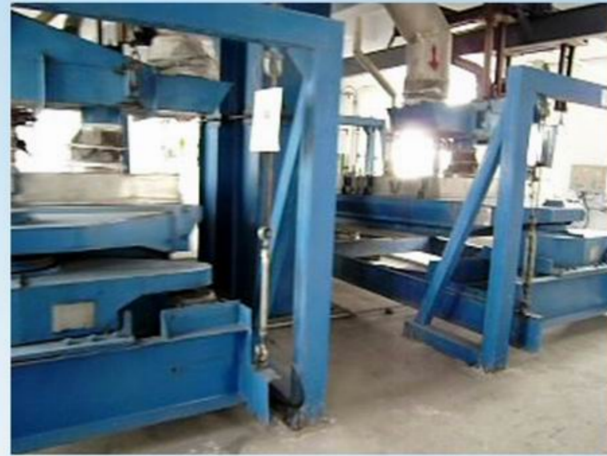
Screener MH-TE36 (Left) For Screening UREA at site
