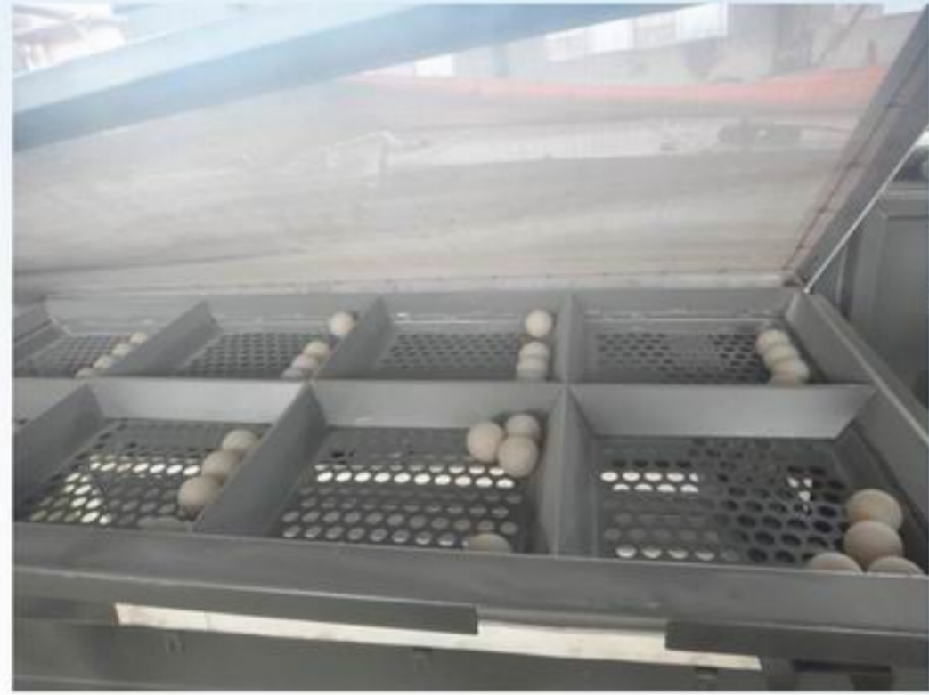
The self-cleaning ball could be rubber , silica gel, Polyurethane, that could meet different industry request.
